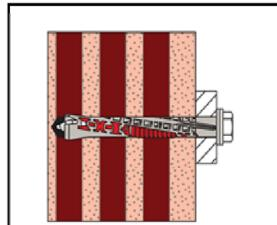
5. Correctly installed anchor.
