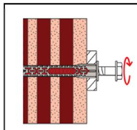
4. The screw is screwed-in until the head of the screw touches the sleeve. The anchor is correctly installed, if the head of the screw fits tight on the surface and nor the anchor sleeve neither the screw cannot be turned-in any further.
