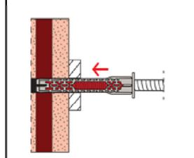
3. Insert anchor (screw and sleeve) by using a hammer until the collar of the plastic sleeve is flush with the surface of the fixture.
