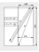
LMB = inside clearance LMH = inside height STB = sliding door width P2 = diagonal clearance LS = running track
