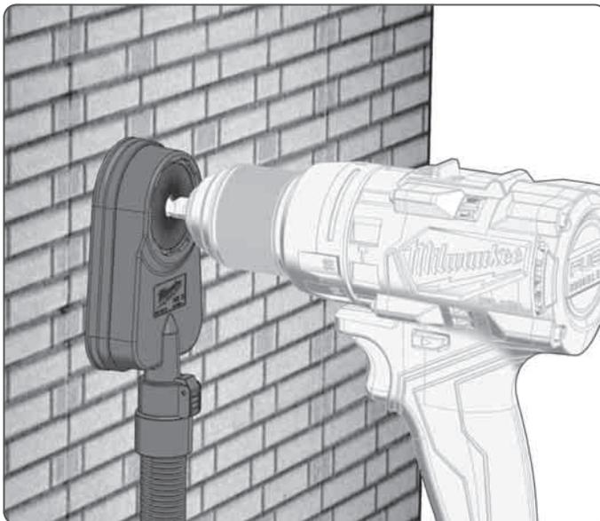
Connect the machine to a suitable dust extractor.
