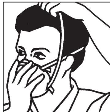
Pull the top strap over your head resting it high at the top back of your head. Pull the bottom strap over your head and position it around the neck below the ears.
