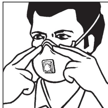
Place the fingertips of both hands at the top of the metal nosepiece. Mould the nosepiece to the shape of your nose by pushing inward while moving your fingertips down both sides of the nosepiece. Pinching the nosepiece using one hand may result in less effective respirator performance.
