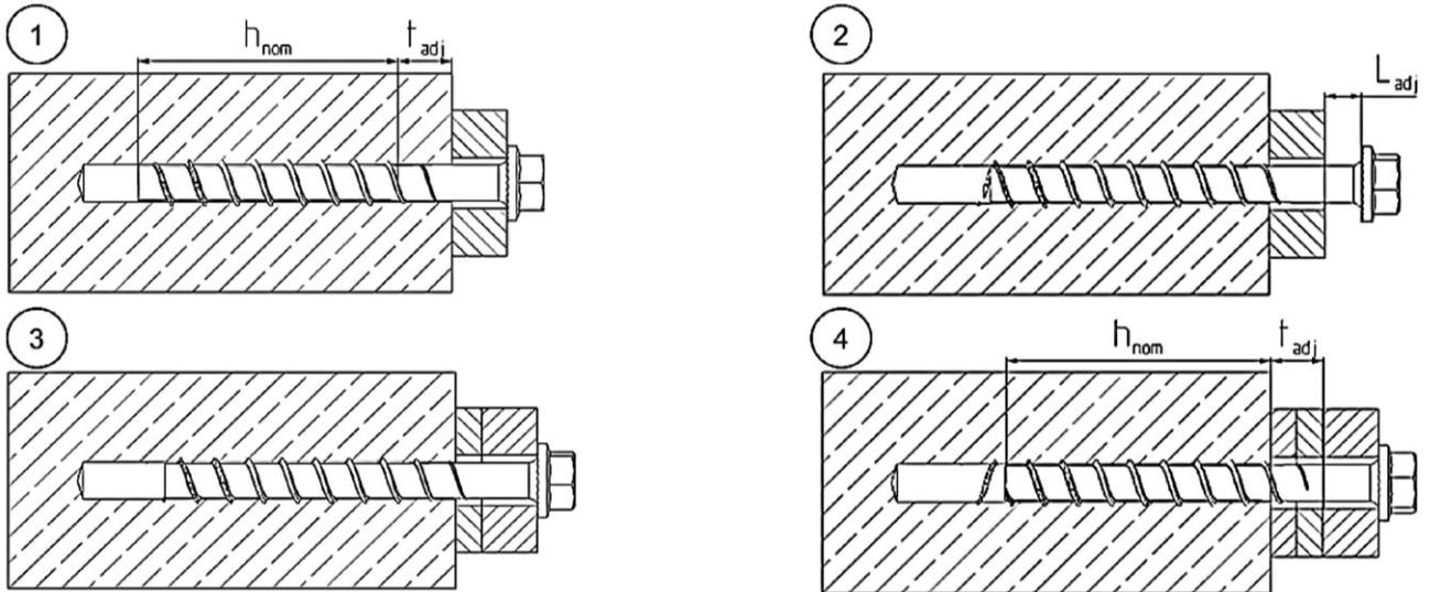
It is permissible to untighten the screw up to two times for adjustment purposes. Therefore the screw may be untightened to a maximum of  $L_{adj} = 20$  mm to the surface of the initial fixture. The total permissible thickness of shims added during the adjustment process is  $t_{adj} = 10$  mm.
